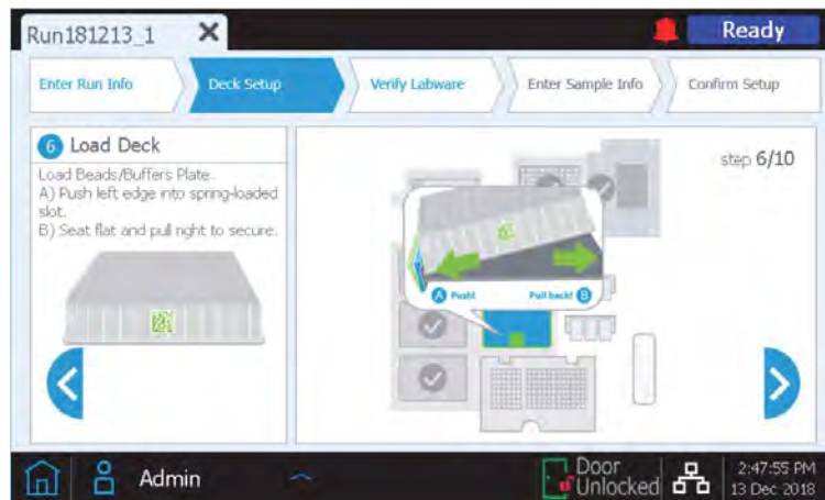
Figure 11. Step 6 of 10 of the Deck Setup screen of the Magnis NGS Prep instrument.
